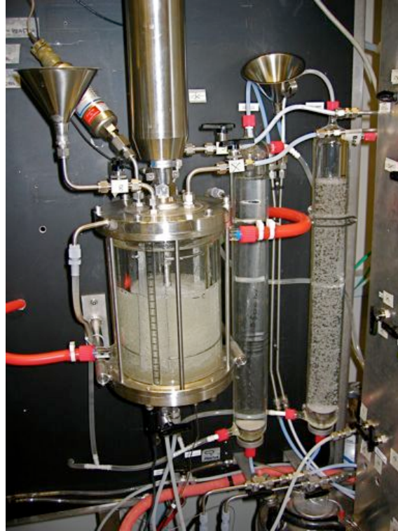
FIGURE 4.1. Photograph of the core of the stirred cell setup in continuous mode
